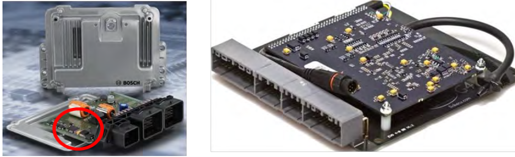
Figure 5: An ECU with tantalum capacitors on board (in red circle) (photos: Bosch (left), Subaru WRC (right))
